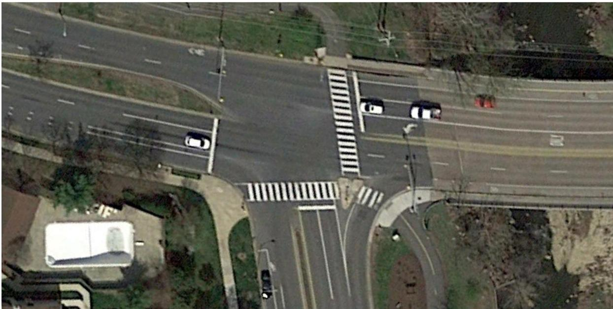
While Arlington County generally tries to eliminate slip lanes, the heavy traffic along AMD makes the slip lanes necessary.
