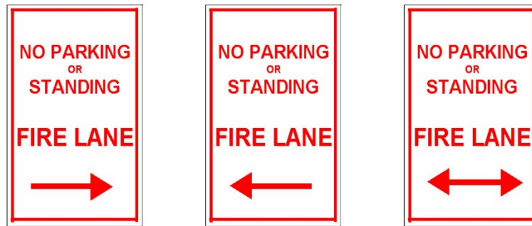
Figure 503.3.2 Fire lane signs
